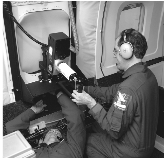
Fig. 2 ECHELLE being mounted at the aircraft window by camera operator Mike Koop (bottom) and the author. Photo: NASA.
